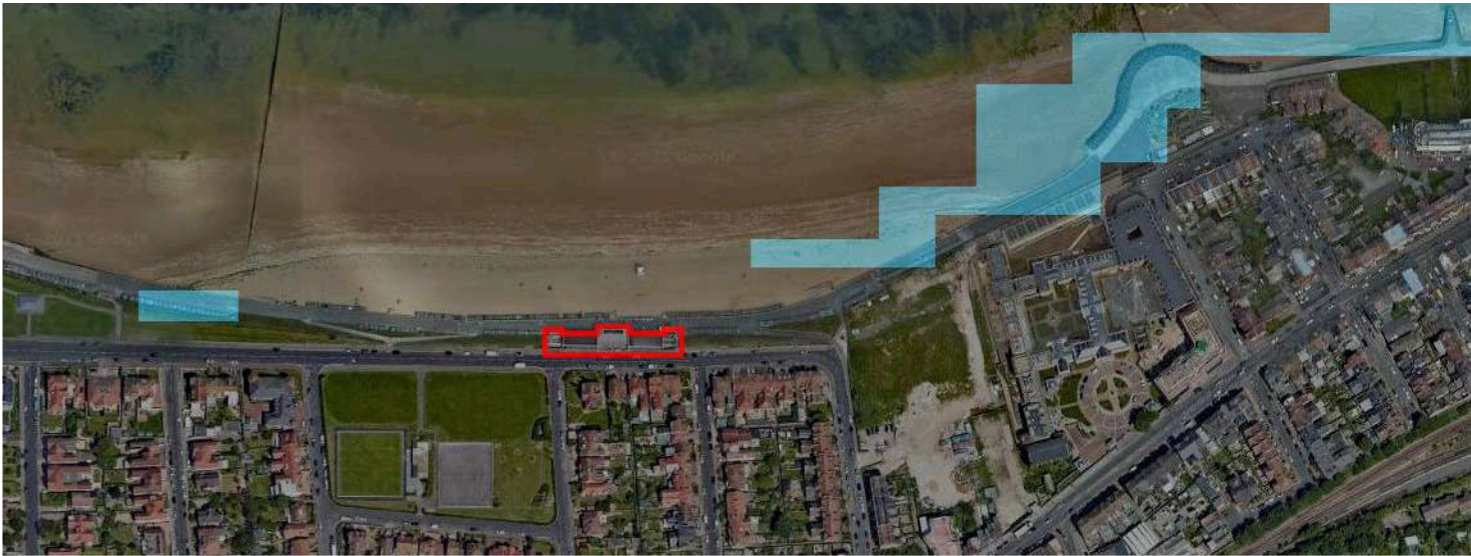
Diagram showing impact of sea-level rise of three-feet. Westbrook Loggia, outlined in red, is unaffected although parts of the promenade are compromised.
